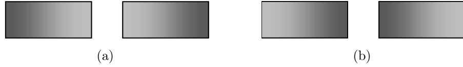
Figure 2.8: Proximity effect from the current flowing in the neighboring lines. (a) Even-mode coupling. (b) Odd-mode coupling.
